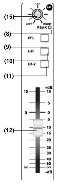
determines the relative amount of left and right channel signals being sent to buses G1, G2 respectively when the **G1-2 Select switch (11)** is engaged.
